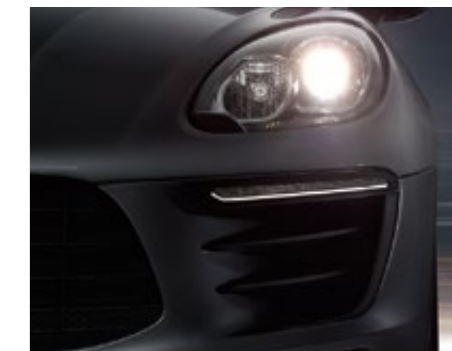
Dipped beam with halogen headlights
