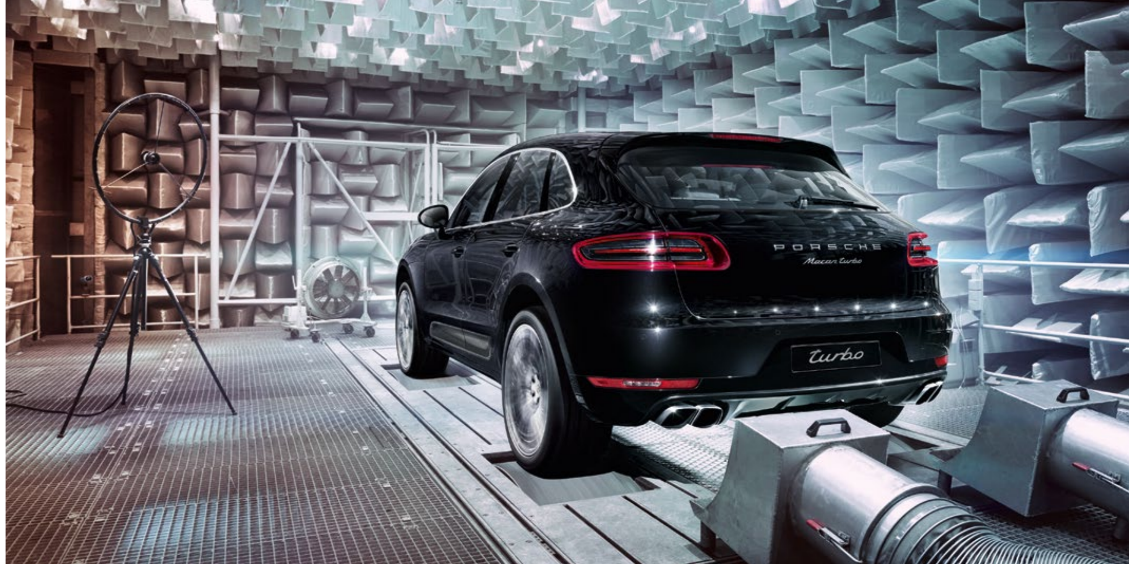
Acoustic test chamber in the Porsche Development Centre, Weissach
